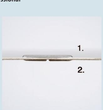
With the new two-stage stapling action, the staple legs pierce the paper first. The staple ends are then bent over and pressed absolutely flat against the paper.
